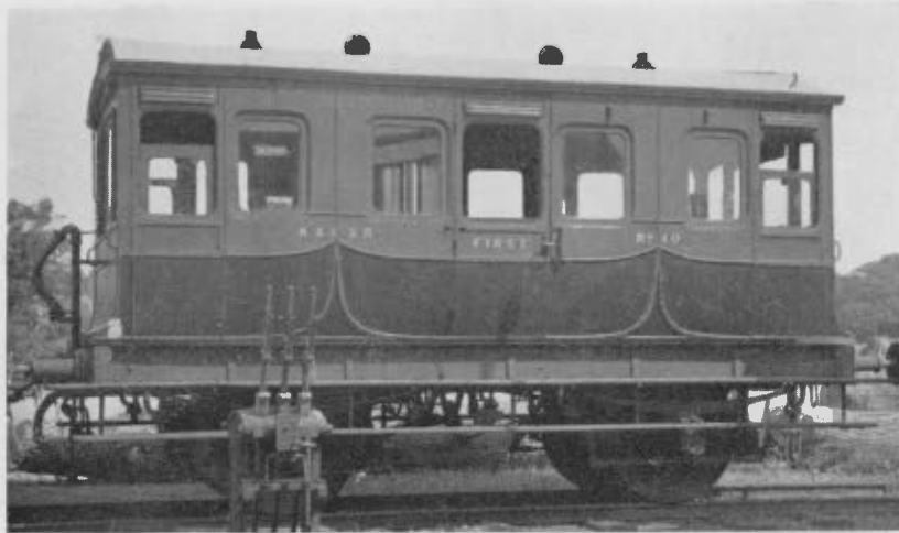
PHOTO H. C. CASSERLEY. 4 wheel Royal Saloon built for L.S.W.R. in 1848. Photograph taken August 19th, 1933.
