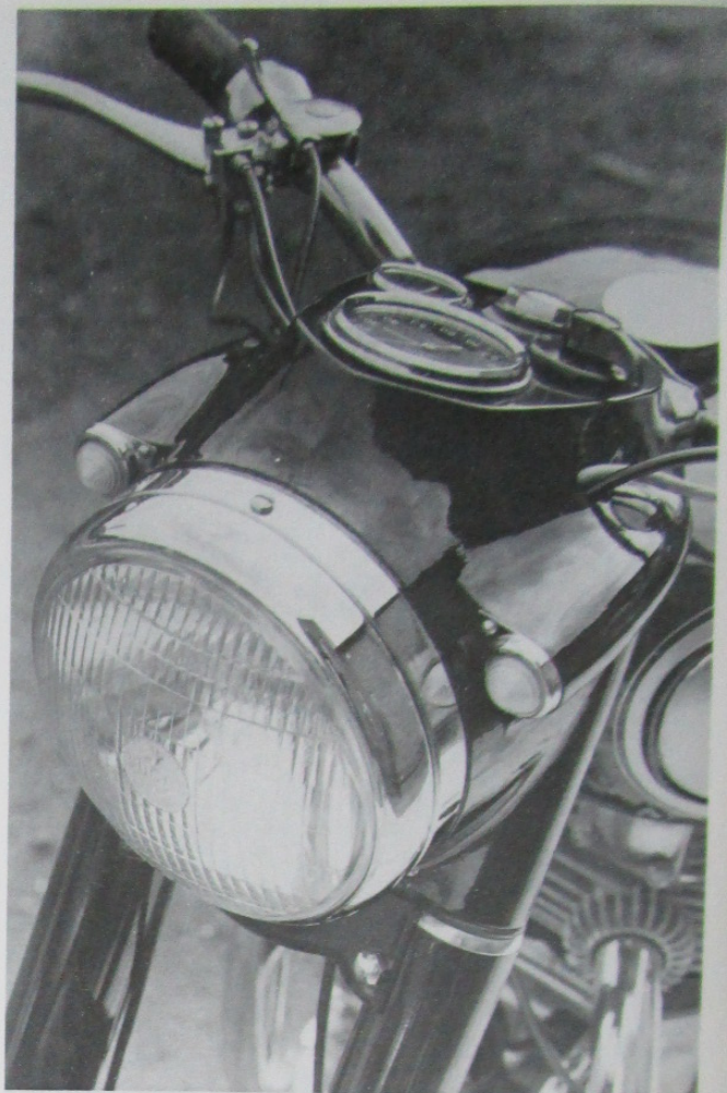
(Top left) Timing chest cover conceals chaindrive to the camshaft etc. Combined oil filler cap and dipstick are by the gear pedal. Sump is dry though oil is contained in crankcase compartment. (Above) The traditional Enfield casquette with its lethal, near-invisible sidelights. (Left) Rear chain enclosure, lengthy and effective propstand, light alloy centre stand and snailcam chain tensioners. (Below) Toolbox and ignition compartments, single Amal Monobloc carburetter and strip-metal cylinder head steady. (Opposite page) This editorial broadside picture is, like all those used here, a genuine roadtest photograph. None are publicity shots. Note length of rear brake pedal
